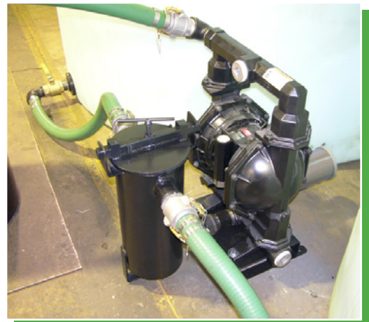
Air-driven dual diaphragm pump (Requires separate air compressor - 30 CFM recommended)
